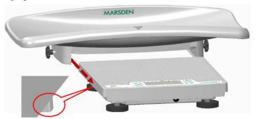
2. Install the tray at the proper location and tighten the screws on both sides.
